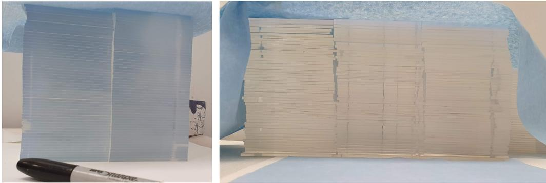
Figure 4.3: The tiles before (left) and after (right) the polishing.
