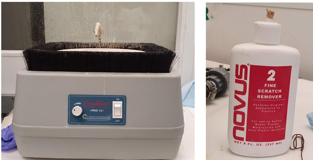
Figure 4.2: The polisher: CrystalMaster Pro 12 Lap Grinder Kit (left) and the NOVUS fine scratch remover (right).
