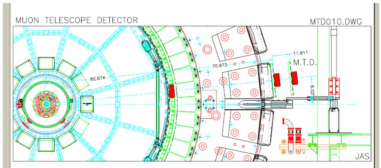
**Fig.11 Engineer drawing of the test MTD**
