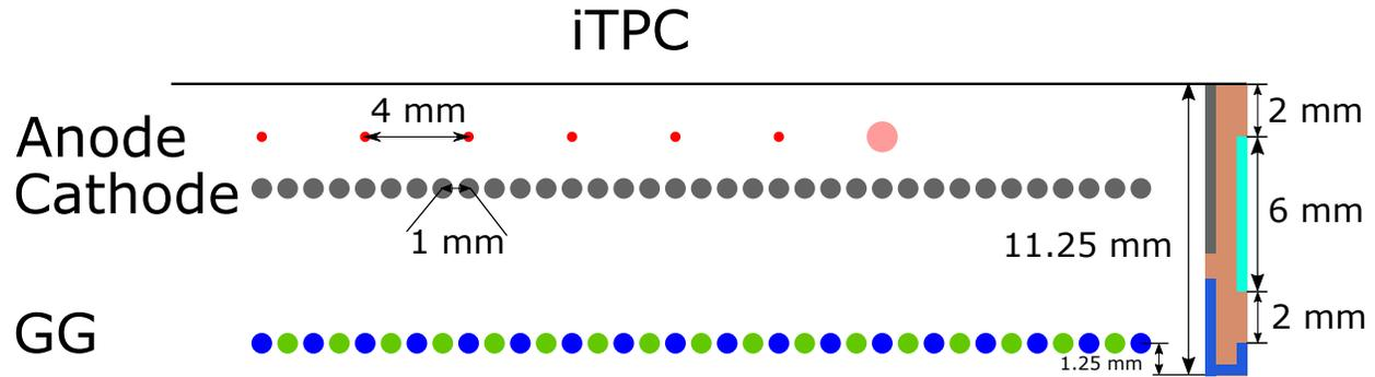
**Fig. 10.** Final wall design for IO region
