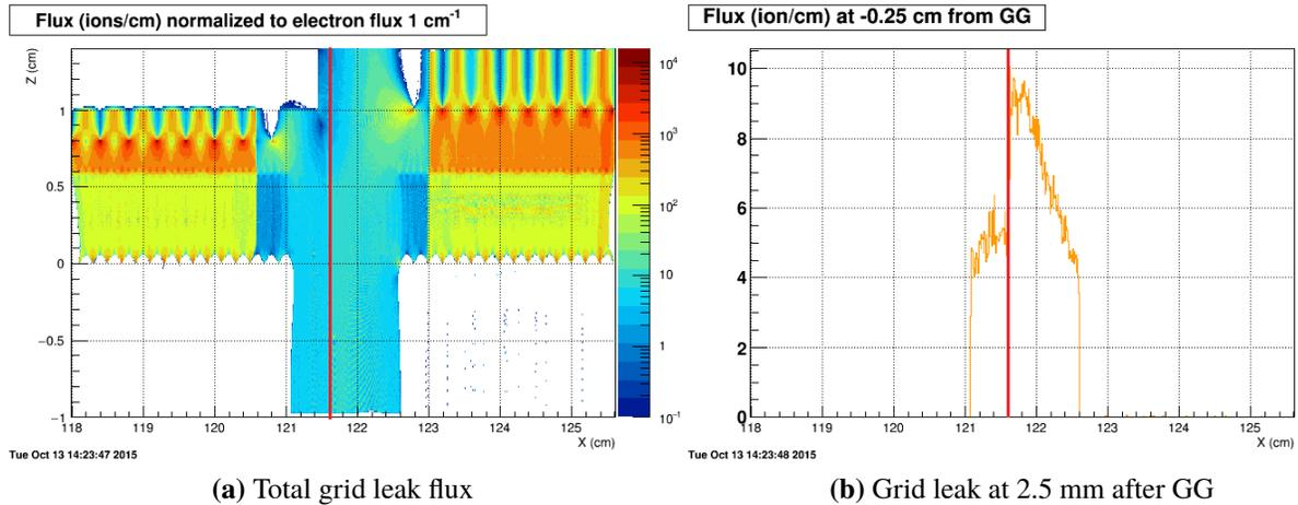
**Fig. 6.** TPC grid leak in IO region with red line indicating the visible border between the leak from the inner and outer sides of the IO region
