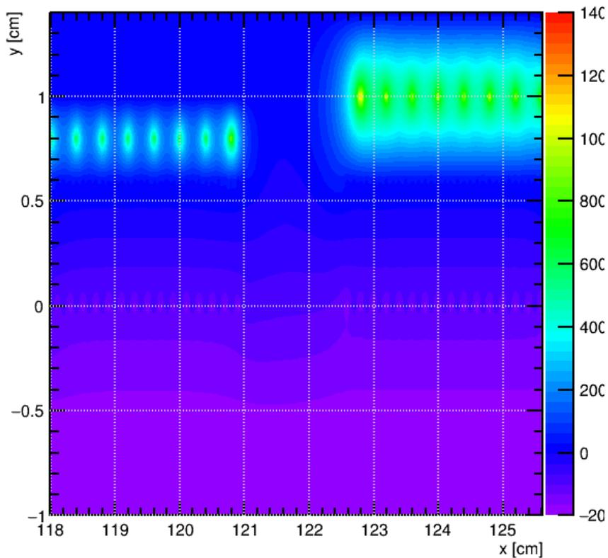
**Fig. 2.** Electric field near IO region of the current TPC setup as simulated by GARFIELD
