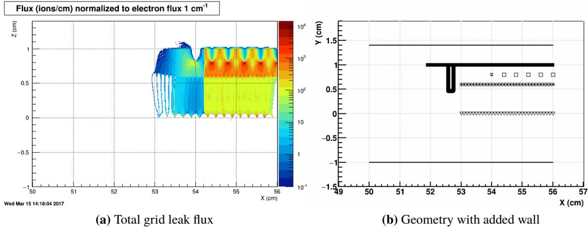
**Fig. 5.** TPC grid leak in II region with additional wall
