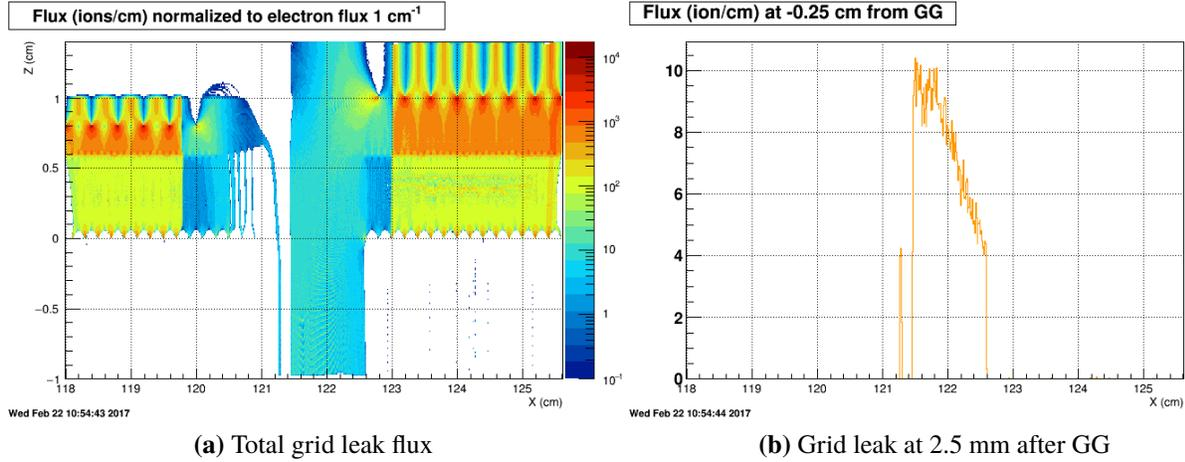
**Fig. 7.** TPC grid leak in IO region with anode wires receded under the the GG by two pitch steps
