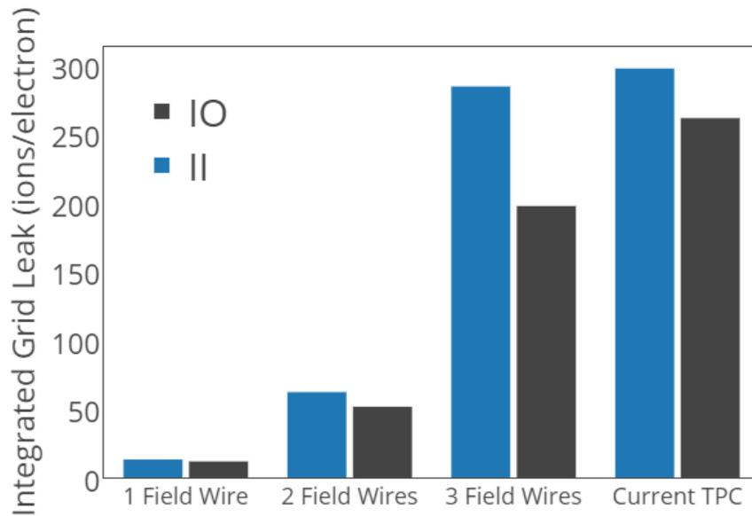
**Fig. 4.** TPC grid leak for different configurations of field wires
