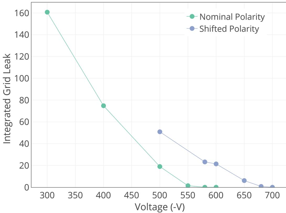
**Fig. 9.** Grid leak as a function of the potential of the outside part of the wall
