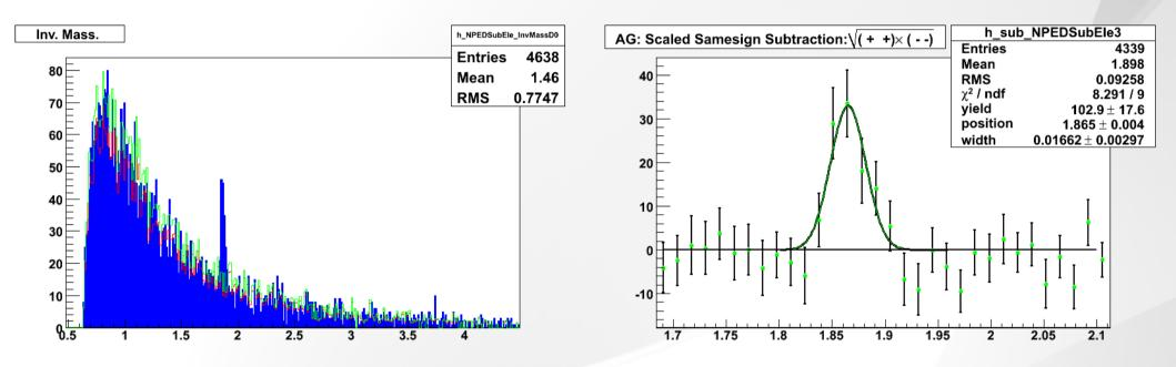
$\label{eq:Fit results} \begin{array}{l} \mbox{Fit results} \\ \mbox{Peak position } m = 1865 \pm 4 \ MeV/c^2 \\ \mbox{Width of the signal } \sigma_m = 17 \pm 3 \ MeV/c^2 \end{array}$
