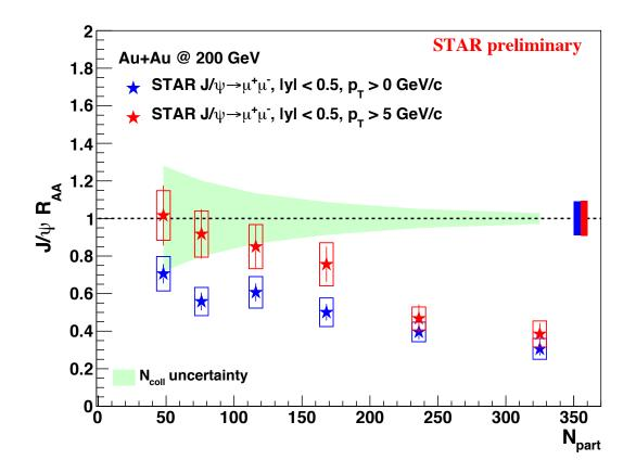
**Central collisions:** significant suppression is observed for both low  $p_T$  and high  $p_T$  (> 5 GeV/c) J/ $\psi$
