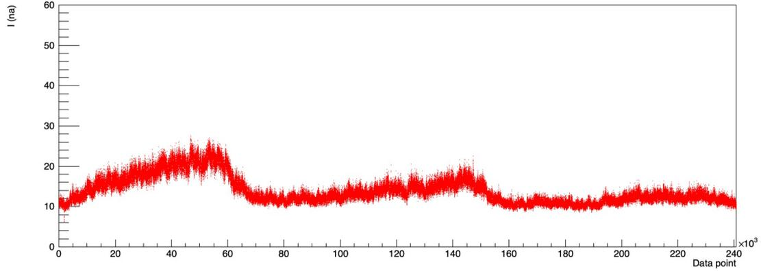
**Figure 3.** The full size prototype's leakage current monitoring at a high voltage of 3200 V.
