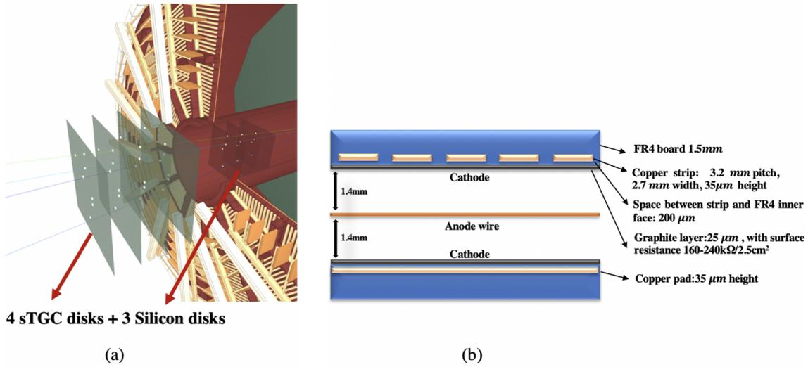
**Figure 1.** (a) The STAR FTS layout side view. (b) Schematic layout of a sTGC chamber.
