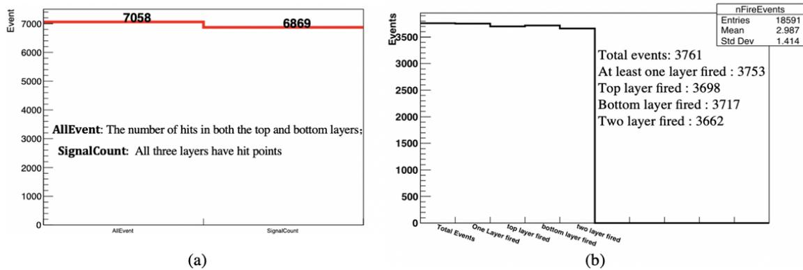
**Figure 7.** The signal coincidences of different sTGC chambers. (a) Full size prototype at 2700 V in cosmic ray test (Efficiency  $>97\%$ ). (b) Pre-prototype at 2800 V during the STAR 2019 data-taking (Efficiency  $>98\%$ ).
