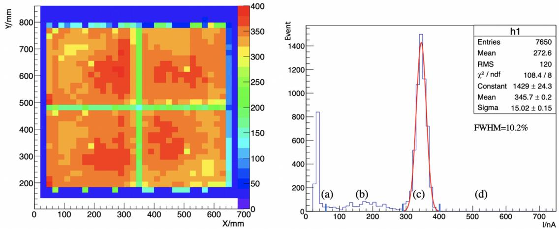
**Figure 4.** The X-ray scan result of the full size prototype chamber. Left: 2D scan result with X-ray scanner. Right: The current distribution during the X-ray scan.
