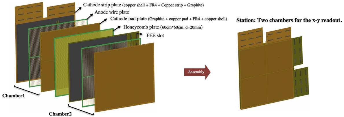
**Figure 2.** Station geometry of full size prototype.
