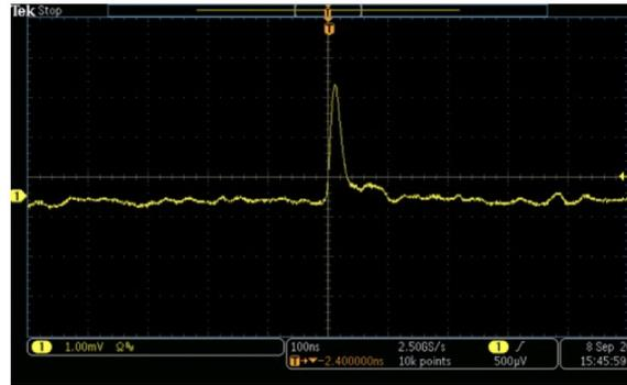
**Figure 6.** Cosmic ray analog signal on a strip. The signal width and amplitude are about 150 ns and 3 mV respectively.
