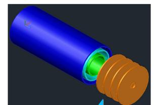
Disk setup used to hold 12 triple GEM segments
