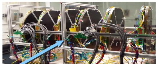
FGT located in the Temple University GEM lab for refurbishing the front-end electronics.
