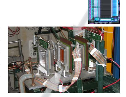
A full APV25-S1 chip readout system has been tested also.
