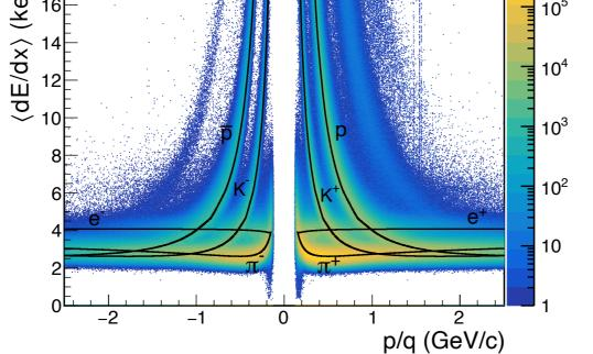
Particle identification is done via <dE/dx> measured in TPC
