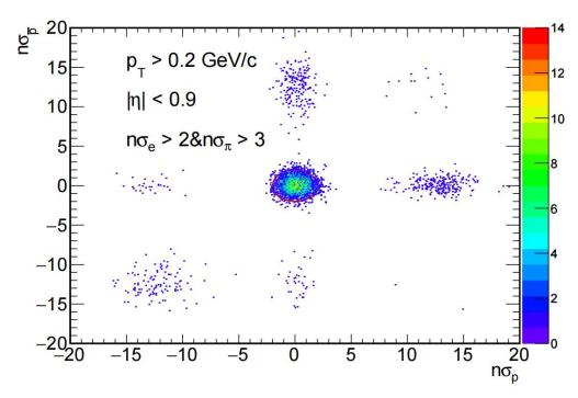
$$n\sigma_x = \frac{1}{\sigma} \log \frac{\langle dE/dx \rangle^{Measured}}{\langle dE/dx \rangle_x^{Theory}}$$
