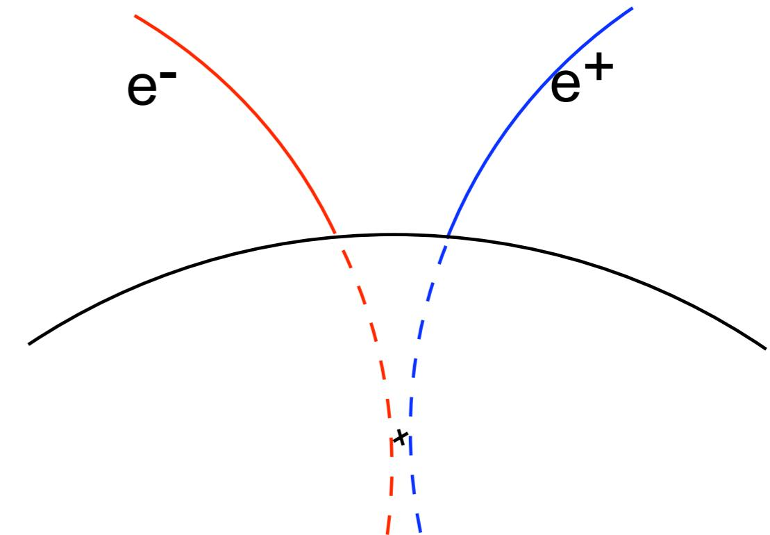
~50% of electrons originating from  $\gamma$ -conversions and  $\pi^0$ -Dalitz decays can be removed with invariant mass method
