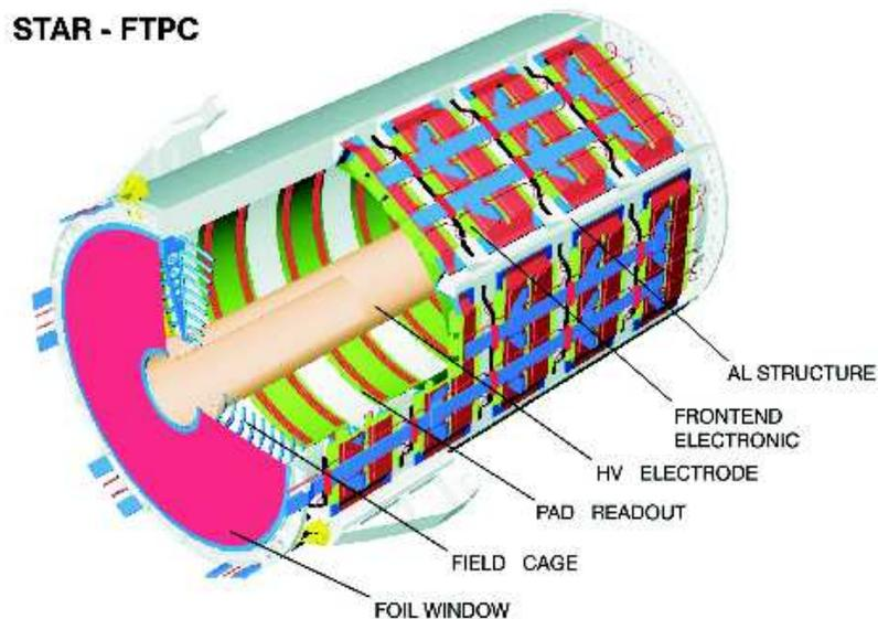
Figure 3.4: Schematic diagram of a STAR FTPC. The figure is from [61].
