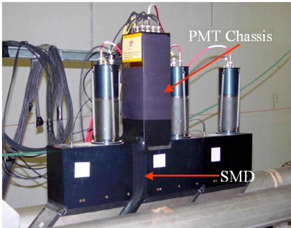
Figure 4.4: A ZDC-SMD module shown installed at STAR.
