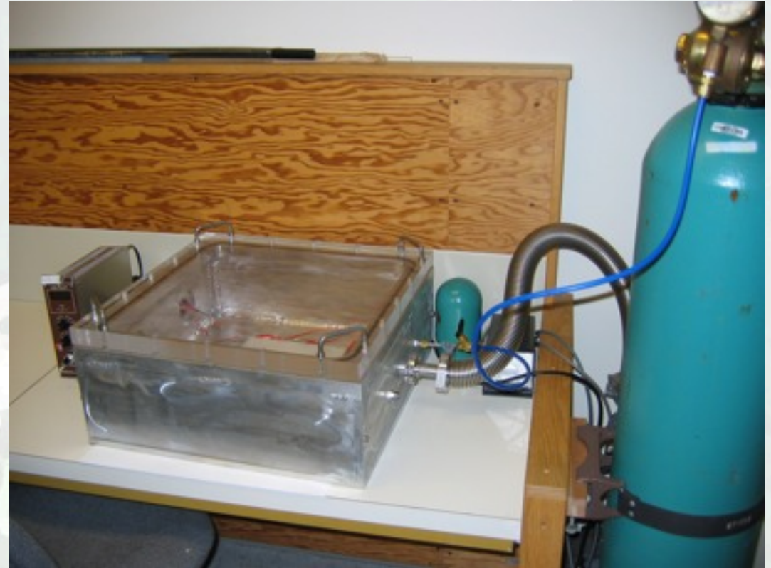
HV Vacuum / Nitrogen box for GEM foil dark current tests
