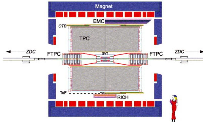
Figure 2.2. An illustration of a cutaway side view of the STAR detector. Figure modified from [30]
