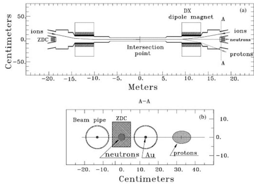
Figure 2.6. The illustration of the Zero Degree Calorimeter at STAR. Figure taken from [35].
