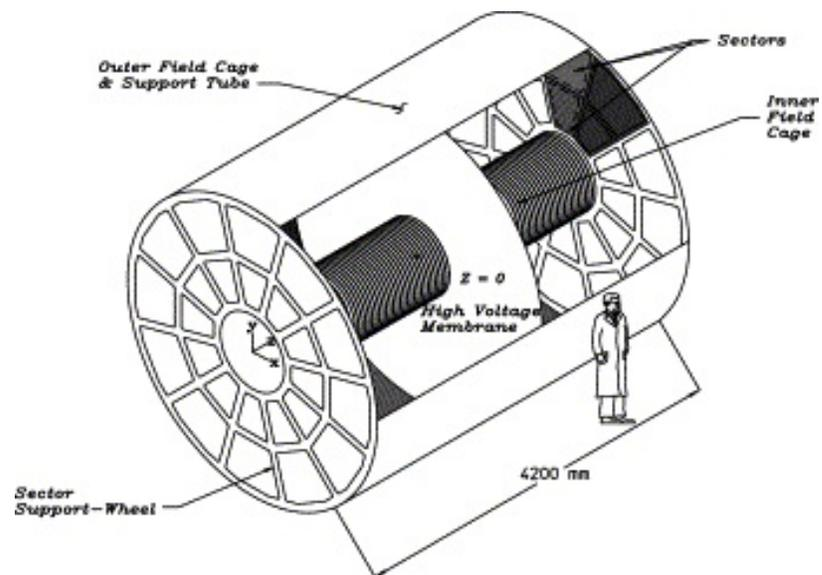
Figure 2.3. The illustration of the Time Projection Chamber(TPC) at STAR. Figure taken from [32]
