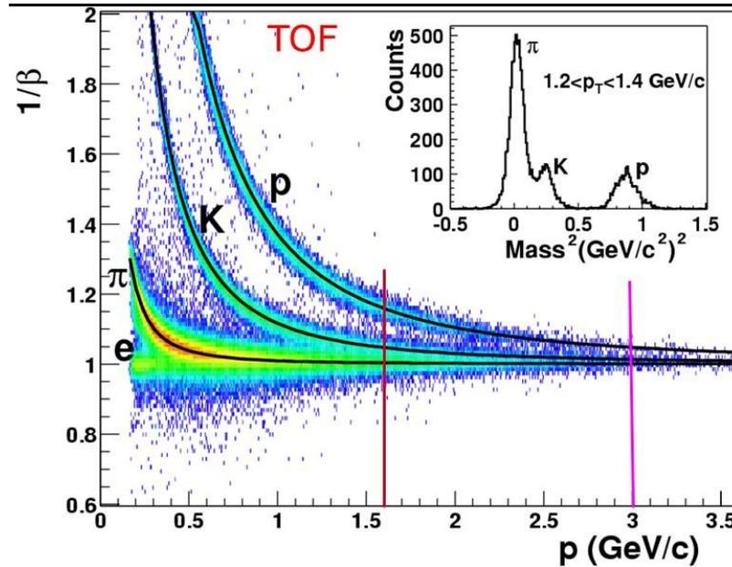
Figure 2.4. Particle identification provided by the Time of Flight (ToF) detector at STAR. Figure taken from [33].
