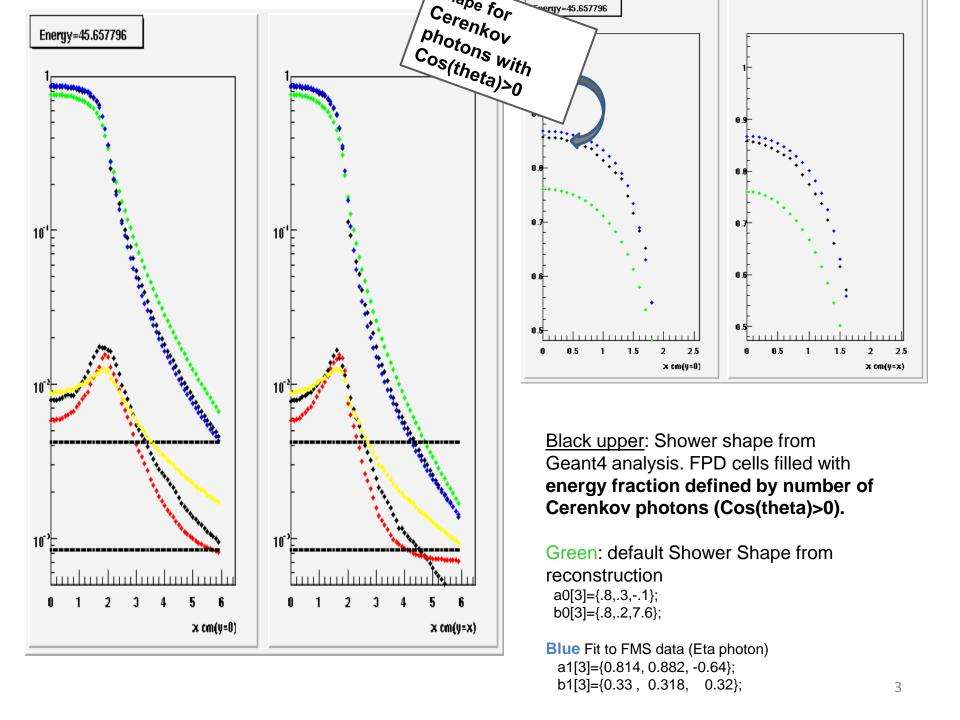
The Cerenkov photons are produced mostly in the forward direction and this leads to enhancement of the high tower cell for photons that strike the center of the high tower cell. The factional change is larger for more forward photons.
