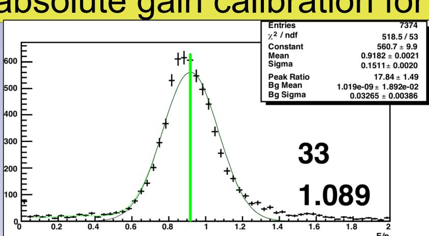
Minimum ionizing particles (MIPS) deposit 200-300 MeV in each tower. The mean of the MIP distribution is used to set the relative gain of towers within an η bin.
