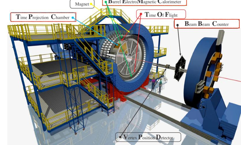
Barrel Electromagnetic Calorimeter (BEMC)
