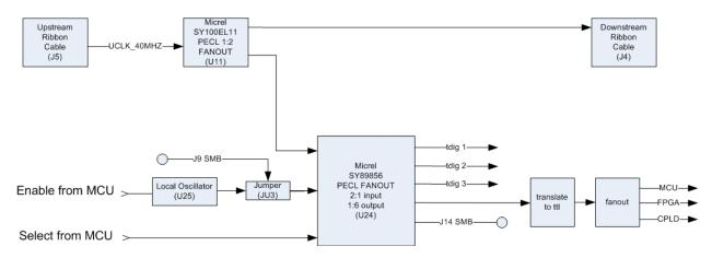
The Upstream input clock UCLK\_40MHZ is buffered and split with U11, one output leg goes directly to the downstream connector. With this arrangement, a failure in the clock switching control will not affect operation of downstream boards.
