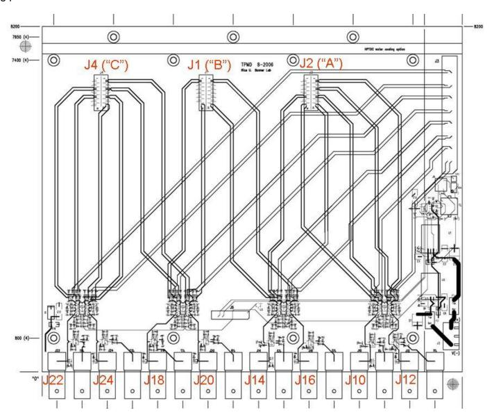
The resulting mapping from the BNC connectors on TPMD to the TDIG connectors and TDIG's HPTDC chips is shown in the following table. There are a total of 8 leading edge mappings ("L.E.") and 8 trailing edge mappings ("T.E.") for each input BNC connector. The leading edge signals are mapped to two HPTDC with 5 channels on U2 and 3 channels on U4, while the trailing edge signals are mapped to one HPTDC (U3) with 8 channels:
