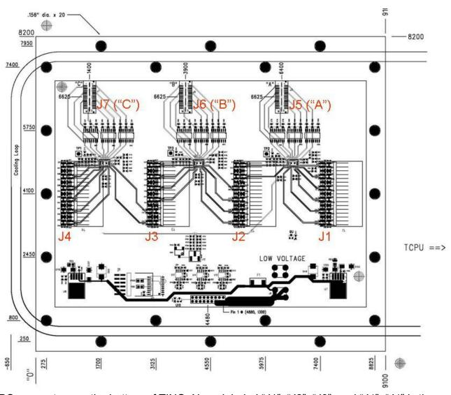
The MRPC connectors on the bottom of TINO\_N are labeled "J1", "J2", "J3", and "J4". "J4" is the connector closest to eta = 0 (away from TCPU), "J1" is the connector closest to eta = 1 (towards TCPU).
