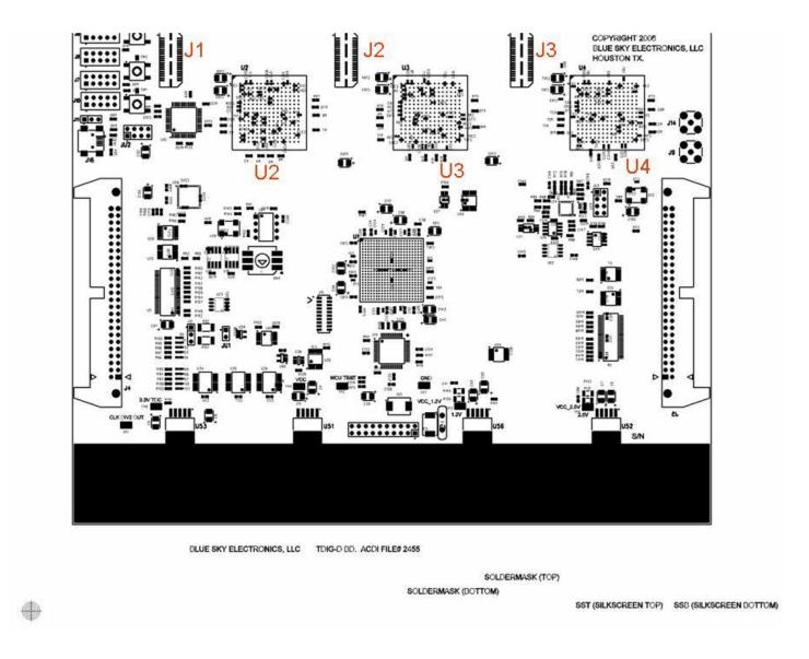
The signal connectors on TDIG-E are labeled "J1", "J2", and "J3". "J1" is the connector closest to eta = 0 (away from TCPU), while "J3" is the connector closest to eta = 1 (towards TCPU). "J1" on TDIG-E mates with J7 ("C") on TINO\_N, "J2" on TDIG-E with J6 ("B") on TINO\_N and "J3" on TDIG-E with J5 ("A") on TINO\_N. TDIG-E has three HPTDC chips on top, labeled "U2", U3", and "U4". "U2" is the chip closest to eta = 0, while "U4" is the chip closest to eta = 1.
