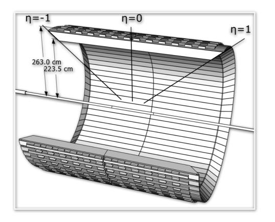
**\***BEMC is a sampling calorimeter and it is segmented into 4800 towers, each with  $\Delta \eta X \Delta \phi = 0.05 \times 0.05$
