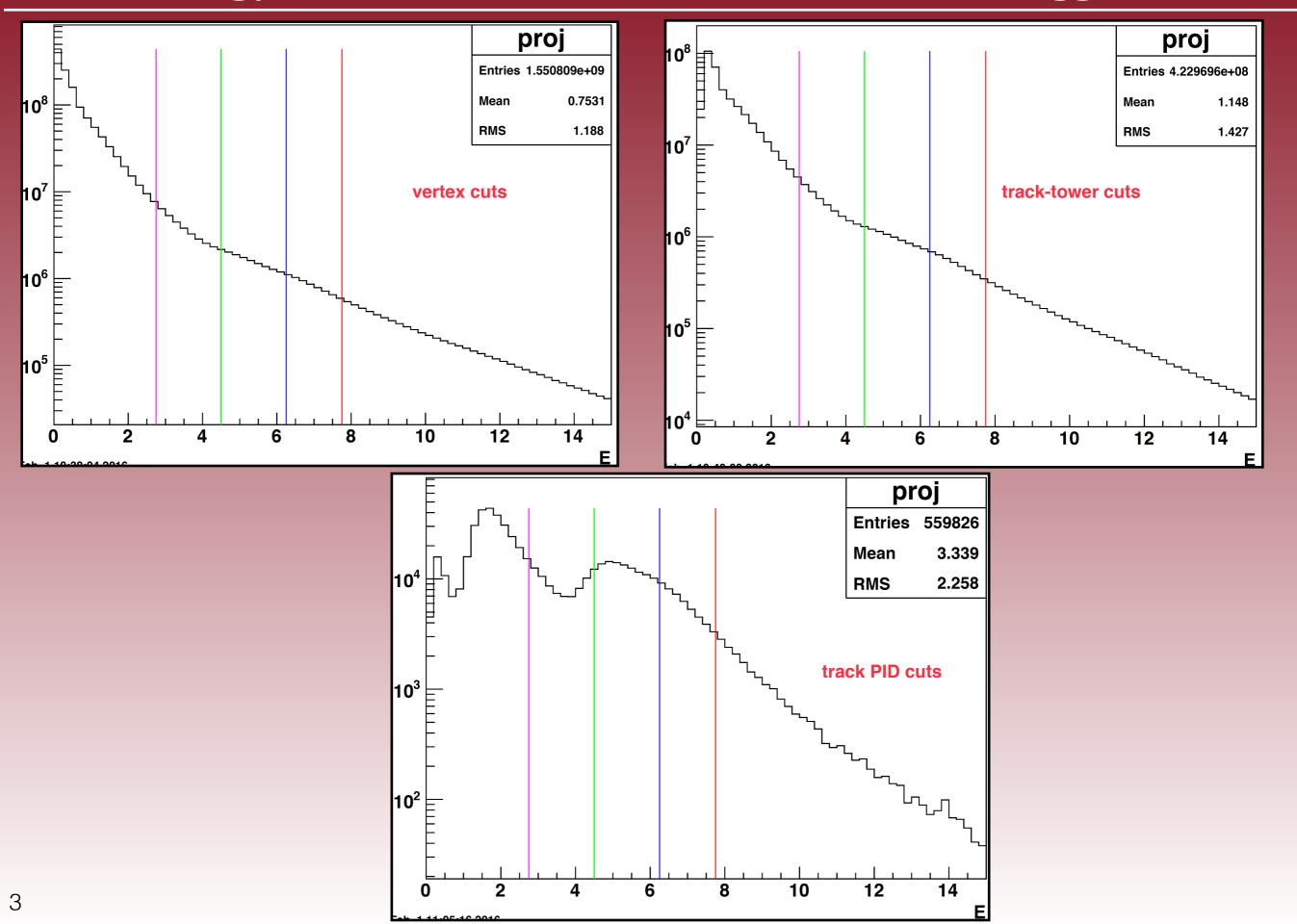
Tower Energy distribution of BHT3->didFire() triggered events where tracks matched to a tower above BHT3 threshold.
