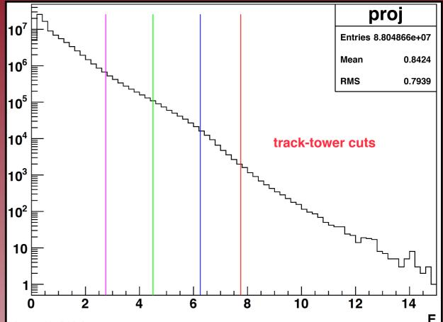
Tower energy distributions of track Matched to a tower above BHT1 threshold
