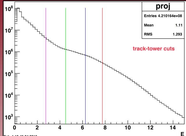
Tower energy distributions of track Matched to a tower below BHT3 threshold
