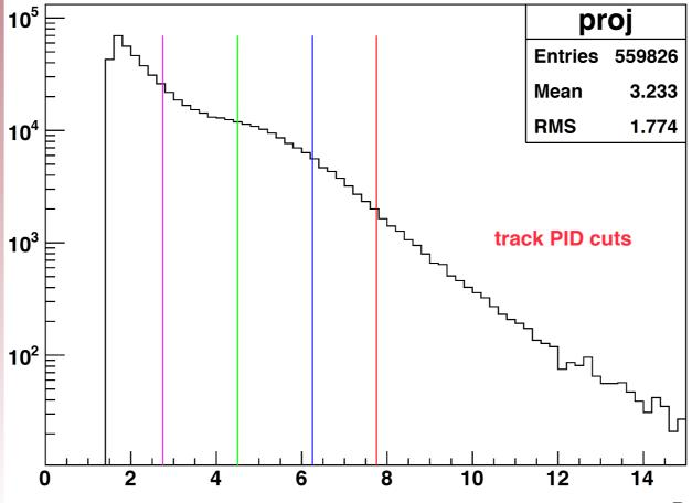
Track Momentum distribution of BHT1->didFire() triggered events where tracks matched to a tower above BHT1 threshold.
