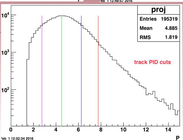
Tower Energy distribution of BHT1->didFire() triggered events where tracks matched to a tower below BHT1 threshold.
