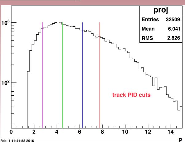
Tower Energy distribution of BHT3->didFire() triggered events where tracks matched to a tower below BHT3 threshold.
