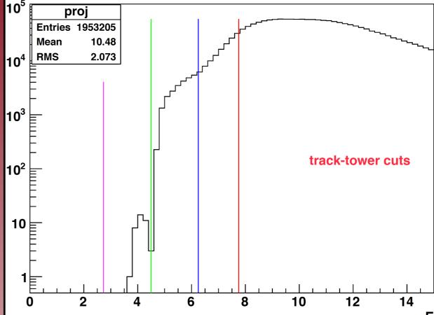
Tower energy distributions of track Matched to a tower above BHT3 threshold
