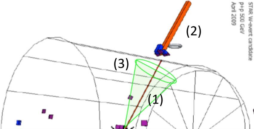
$E_T^{\Delta R < 0.7}$  and  $E_T^{\Delta \phi \sim \pi}$  are formed with track momentum and EMC tower energy ( $p$  of particles reconstructed in detector)
