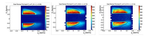
Figure 3.5: East RP track  $p_X$  and  $p_Y$  distributions for three East RP track  $\xi$  ranges. The black curves indicate the ranges of accepted East RP track  $p_X$  and  $p_Y$  cuts.
