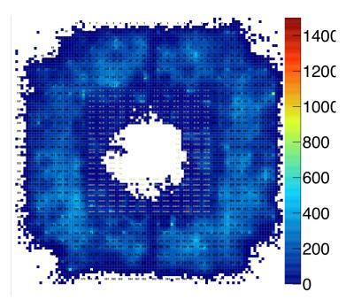
Figure 2.1: Example of EM-jet distribution at FMS before additional hot channel masking. The red color area in this plot indicates the possible hot channels.
